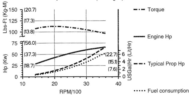
Westerbeke recommends a propeller that will allow the engine to turn 3500-3600 RPM underway at full throttle
